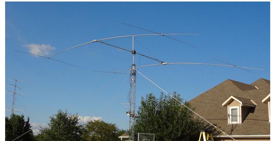
JK402T 2-ele "T" cap loaded Top-rotating & fixed EU
