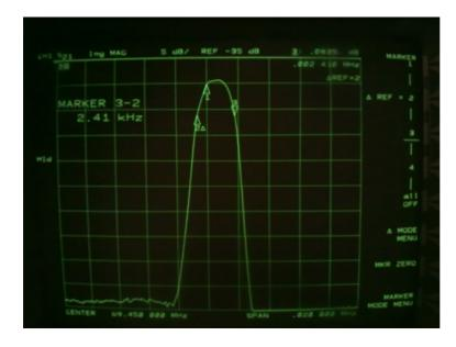
centre freq: 69.450 MHz horiz: span 2 kHz/div reference value: -35dB vert: 5 dB/div
