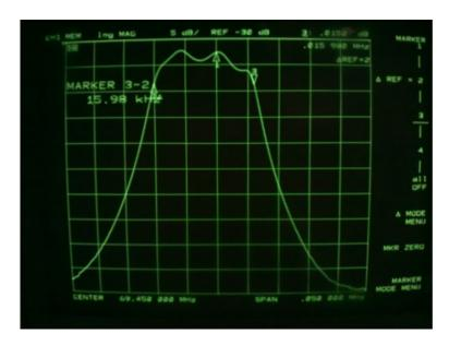
centre freq: 69.450 MHz horiz: span 5 kHz/div reference value: -30dB vert: 5 dB/div
