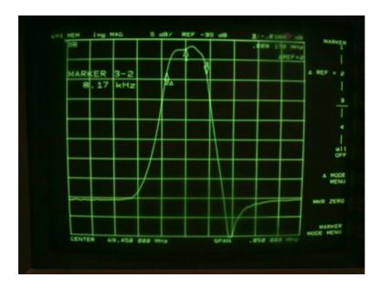
centre freq: 69.450 MHz horiz: span 5 kHz/div reference value: -35dB vert: 5 dB/div
