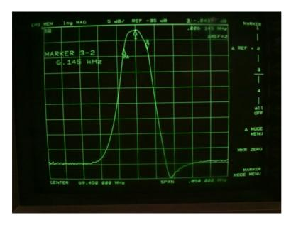
centre freq: 69.450 MHz horiz: span 5 kHz/div reference value: -35dB vert: 5 dB/div
