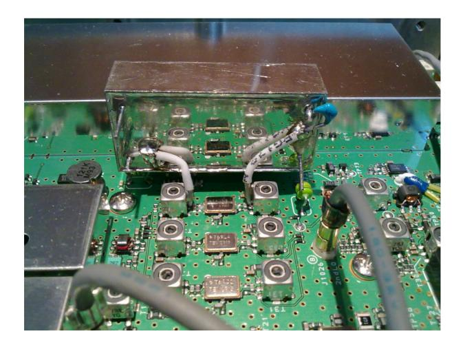
The picture shows the modified section of the main pcb of the FT-950.
