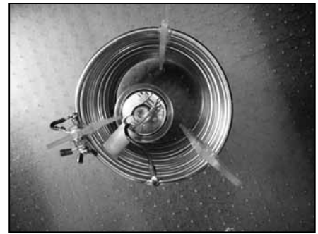
Figure 8 — An 80 meter trap made with 1/4 inch copper tubing wound on a 5 inch form and fixed-value 15 kV surplus vacuum caps
